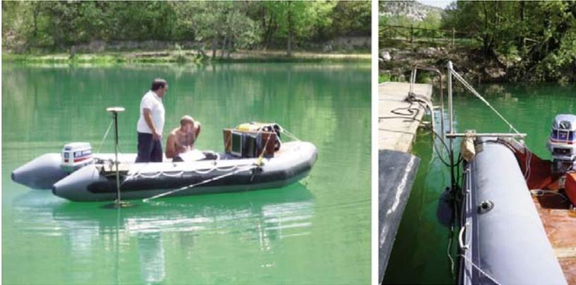
Fig. 12 - The rubber boat "Bombo" equipped with the 8101 multibeam system.
