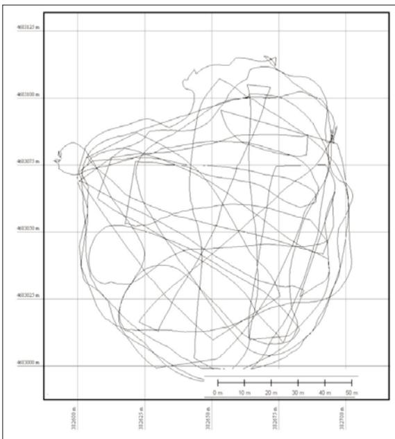
Fig. 13 - Navigation plan for the Sinizzo Lake bathymetric survey.
